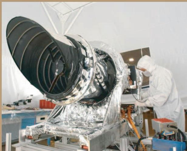
Picture of the HiRISE camera as it is being built by an engineer at Ball Aerospace & Technology Corp. Photo credit: NASA/JPL/Ball Aerospace
